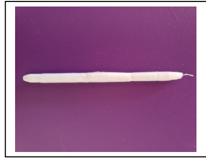
Figure 2: Homemade stylus using a staple rolled into paper.
