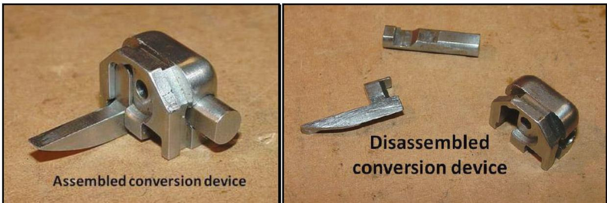
21. A switch can be installed with little technical knowledge in approximately one minute by substituting it for the original slide cover plate, as shown below:
