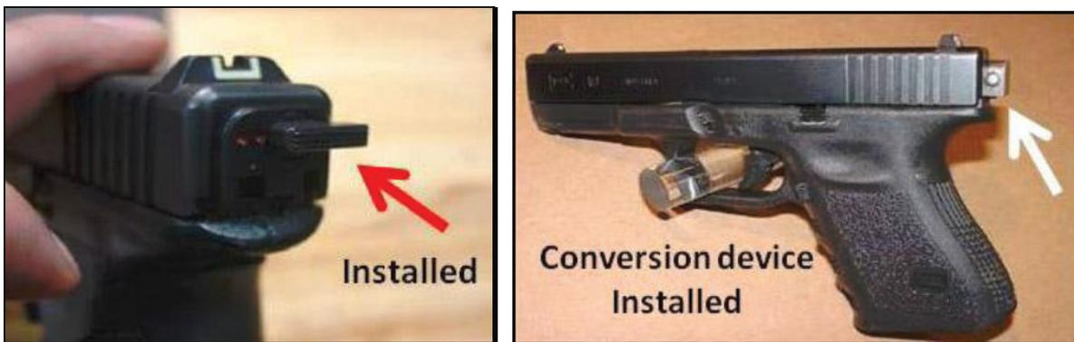
22. When a switch is installed on a pistol and the trigger is pulled, the pistol will fire until the trigger is released or the magazine is empty. A Glock pistol affixed with a switch can fire over 1,000 rounds per minute.
