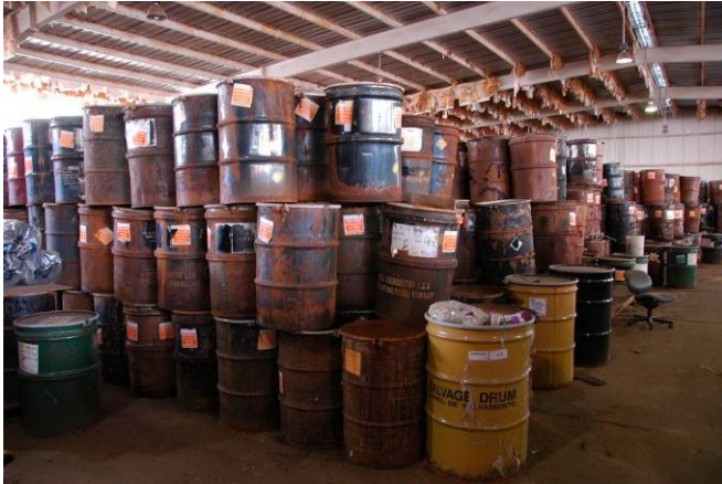
Leaking and corroded drums of KOH waste
