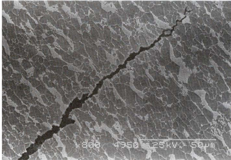
Figure 4-9 Transgranular Cracking in Pipeline Steel (Revie 2000)
