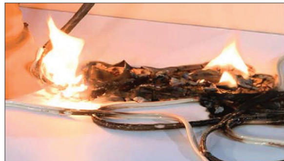
FIG. 22: Overheated Counterfeit Extension Cord.
