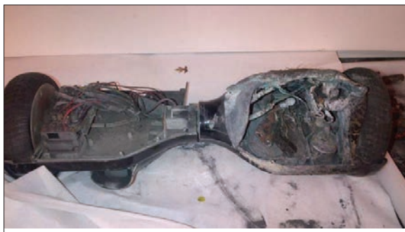
FIG. 23: Overheated Counterfeit Hover Board.
